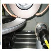
Unison's Model 9100 Pulverizer Blade Regrinder is a 5-Axis turnkey grinder featuring an integrated 25 horsepower, direct drive, dual ended spindle. The direct drive spindle motor provides a continuous torque rating through its entire operating range.
